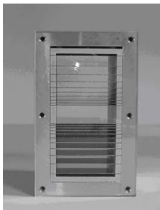
Fig. 14: Test module for tests performance of glass foils vs. shaped Si wafers. Test elliptical Kirkpatrick-Baez optical system, focus 0.5 m, 58 x 50 x 100 mm, glass foils 40 x 40 x 0.3 mm, Si wafers 40 x 40 x 0.4 mm.
