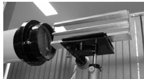
Fig. 16: Optical test of experimental KB system (dimension – 108 mm x 320 mm x 50 mm, glass foils – 100 mm x 300 mm, focus 0.6 m).
