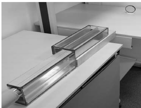
Fig. 15: Test parabolic KB X-ray imaging system based on parabolically shaped glass foils with dimensions of 300 x 100 x 0.3 mm. The complete KB
