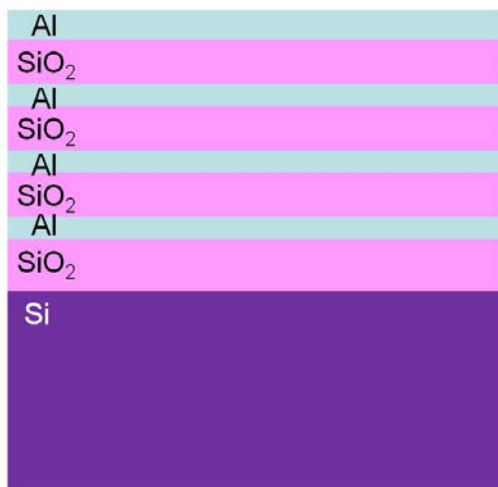
Figure 2. Thin films stack illustration of a traditional Al – SiO 2 bond pad within the pad window. Barrier and other layers are omitted for simplicity.
