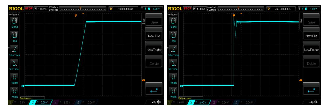
The eFuse (left) has a controlled and adjustable slew rate, reducing inrush current. The relay (right) produces noise and chatters, resulting in power loss.
