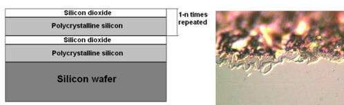
POLY layers enhance the gettering capability of a semiconductor wafer by about two orders of magnitude (measured by MCC) and it is efficient for gettering of heavy metals. However, after each high temperature annealing during the device fabrication process POLY layers losses a great part of its gettering capability.
