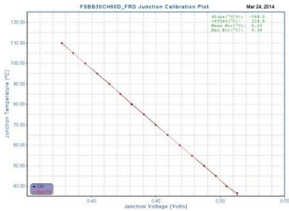
Figure 10. Results of Device Junction Calibration for FRD
