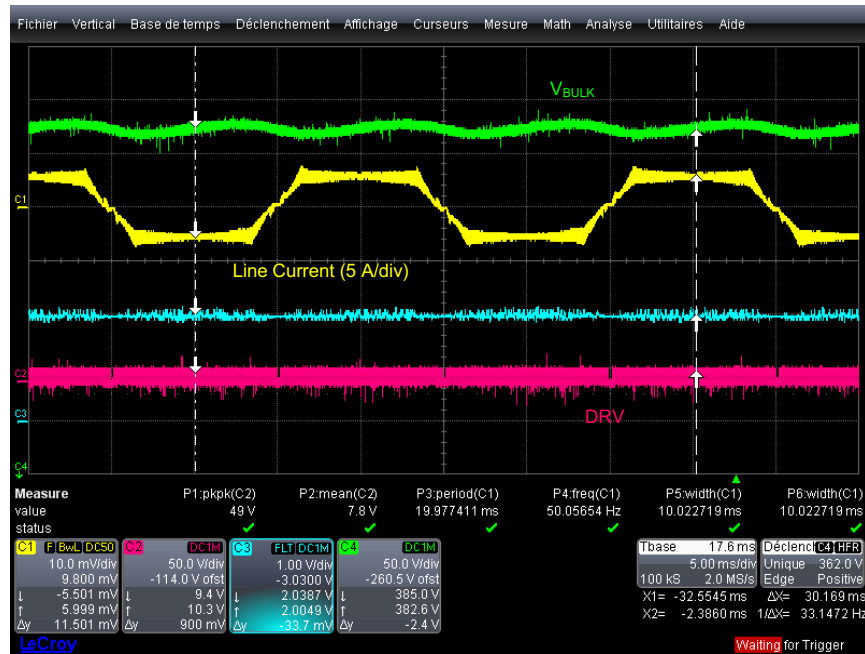
Figure 14. Over-Current Situation (85 V, 0.5 A Load Current)
